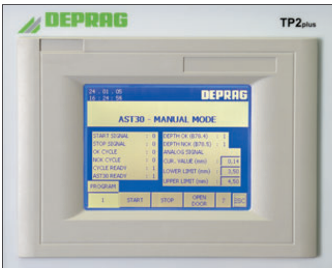
Example for manual mode showing different signal status.
